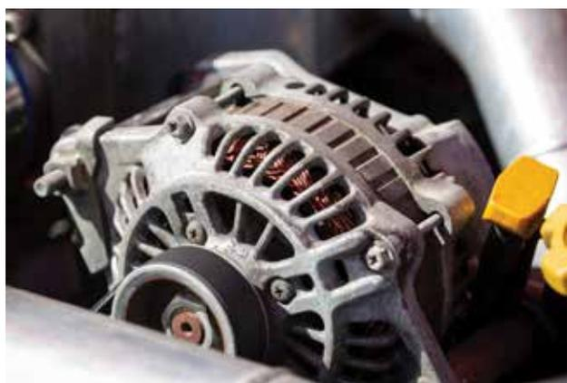
is not working properly. For example, the radio, lights, and automatic windows are powered directly from the alternator in most vehicles. If the alternator is faulty, the battery will discharge very quickly, almost in the course of driving.
